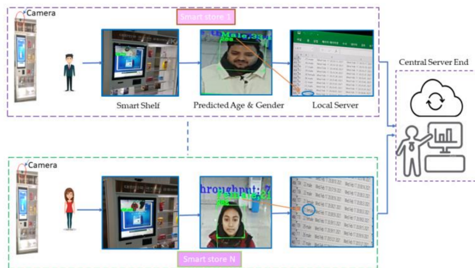
Figure 2. The process diagram of a smart store customer relationship management system.
